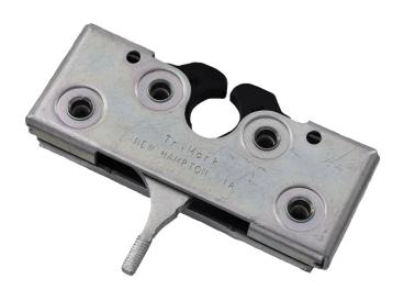
This two rotor latch is a sub-platform to the Tri*Mark* proven 050-0100 series latch and is designed for medium to heavy-duty applications for on or off highway compartments and access panels. It features an internal trip mechanism for applications where it is desirable to have the release mechanism in-line with the latch.
